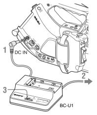
Connect the DC power output cable of the BC-U1/U2 to the DC IN connector of the camcorder.
